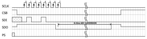
Figure 11: Conversion out sequence, Typ=d1, OSR = 4096
