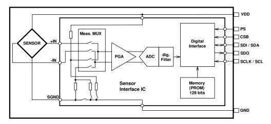
Figure 1: Block diagram of MS5803-01BA
