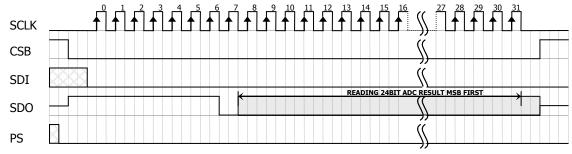
Figure 12: ADC Read sequence
