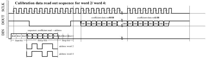
Fig. 6d: W2, W4 READING sequence
