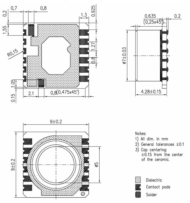
Fig. 9: Device package outlines of MS5534-CM
