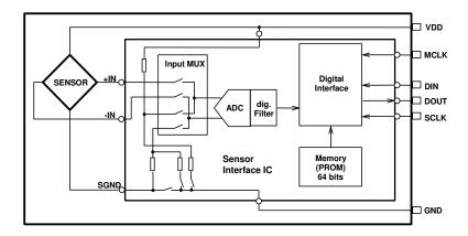
Fig. 1: Block diagram MS5534C
