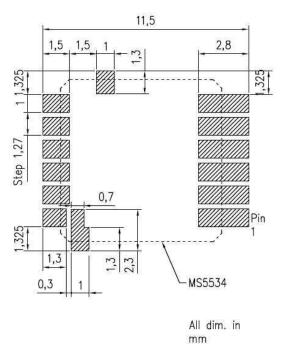
Fig. 10: Layout for bottom side
