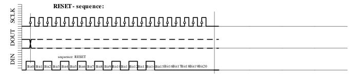
Fig. 6e: RESET sequence (21 bit)
