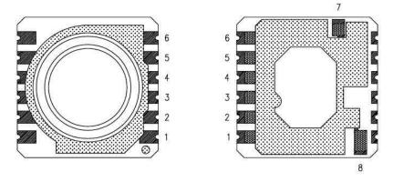
Fig. 2: Pin configuration of MS5534C
