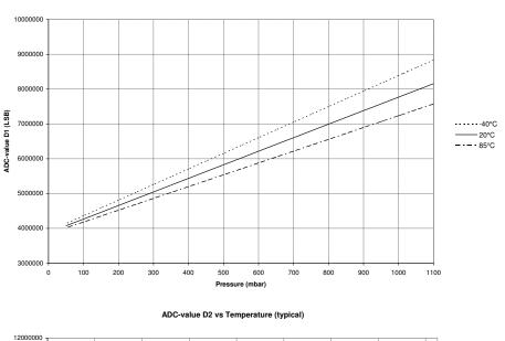
ADC-value D1 vs Pressure (typical)
