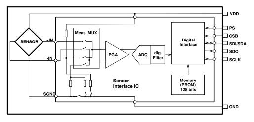
Figure 1: Block diagram of MS5611-01BA
