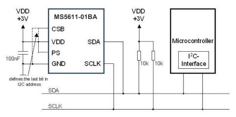
Figure 17: Typical application circuit with SPI / I<sup>2</sup>C protocol communication
