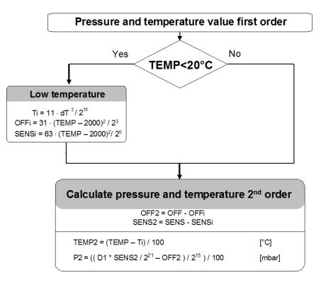
Flow chart for pressure and temperature to the optimum accuracy
