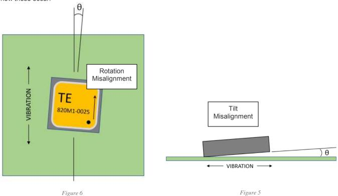
Both types of misalignment result in incorrect output voltages for vibration amplitude. The output error will be proportional to the cosine of the error angle  $\theta$ .
