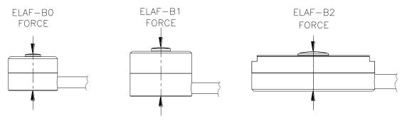
BO, B1 & B2: SPHERICAL CONTACT ON THE TOP AND FLAT SURFACE ON THE BOTTOM
