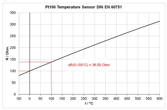
Figure 1: Resistance characteristics
