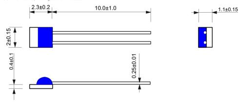
Figure 3: Mechanical dimensions PTFC outline
