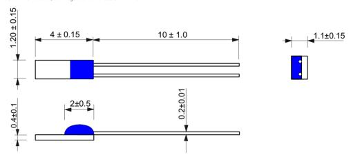
Figure 6: Mechanical dimensions PTFM outline
