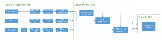
The sensor temperature is calculated using the quotient of the NTC resistance and a fixed reference resistance network. The thermopile voltage is amplified using a low noise high gain amplifier before conversion. All analog signals are converted using the same ADC therefore a multiplexer is used to switch between the different signal inputs. This multiplexer is not shown in the chart.
