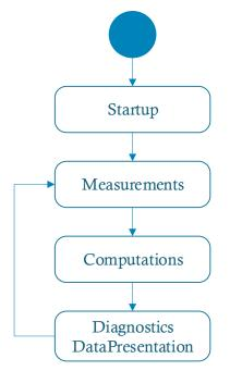
During startup the sensor checks if the data stored in the EEPROM are valid. If no the sensor will response with an error message. See chapter **Diagnostics** for details. When passing the validation, the data are loaded to work RAM. This includes routing of analog frontend, calibration parameters and the serial number. Since there is no read access to the EEPROM data during normal mode allowed this is necessary to read out the serial number during measurements.
