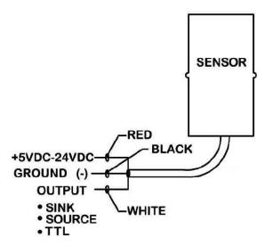
Figure 3: Wiring diagram for SL-630 series elements.
