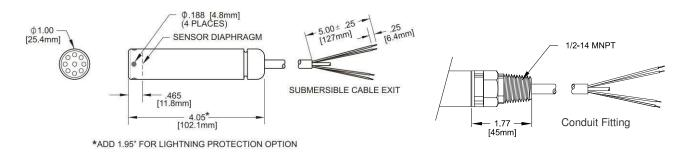
**Gland Cable Seal Configuration for ETFE Cable**
